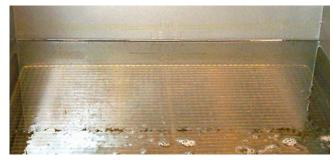
Add fresh shortening until the level is at the top OIL LEVEL line. DO NOT OVERFILL THE FRYPOT.
